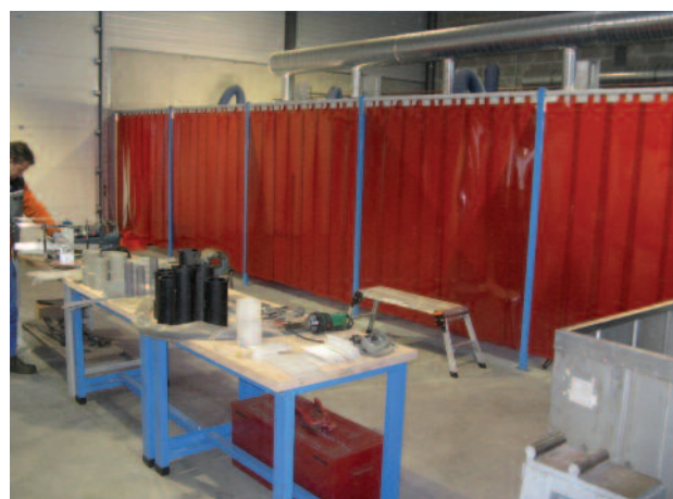
Booths closed with strips (300 mm x 2 mm) 33% overlap.
